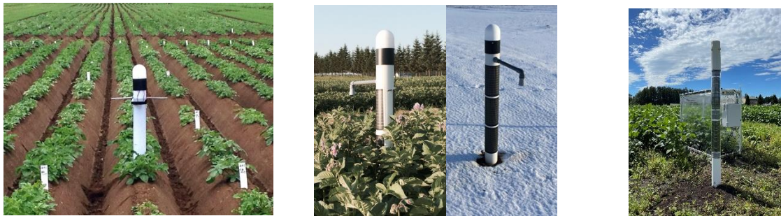
(1) Four 2W-solar panels (2) Three 3W-flexible solar panels (3) Two 3W-flexible solar panels
