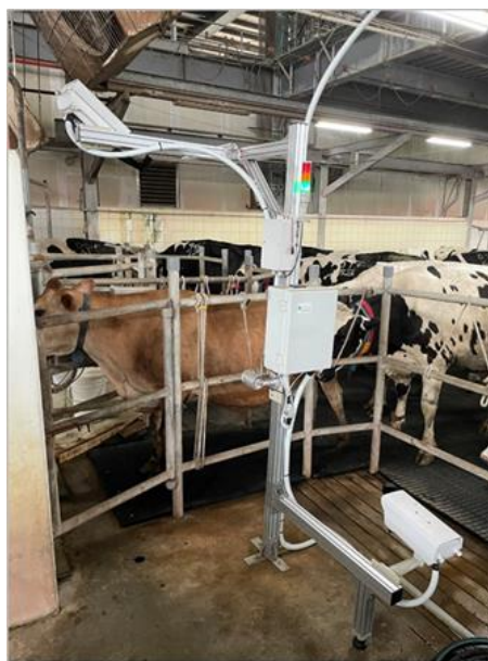
Figure 1. The dual-lens IRTs installed at the milking entrance and automatically measured the temperature of the eye sockets and udders.
