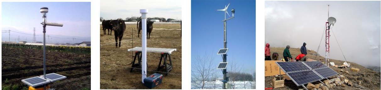
(1) Installed with a pole (2) Installed on a desk (3) With a wind turbine (4) Installed in Himalaya (6500m)
