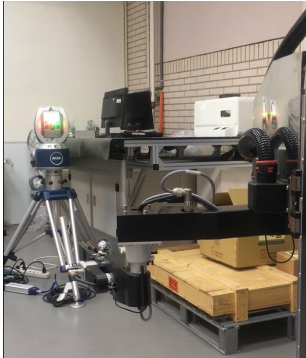
Figure 3. The repeatability measurement tested by laser tracker
