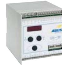
LIS-SV: this load indicator system offers all the functions of the LIS-SE system, but uses load measurement sensors in addition to motor current measurements. This system is an attractive proposition for systems with several hoists where the overall total load of all hoists needs to be limited. This system increases measurement accuracy. The load can be indicated either on the display in the pendant control or on a large load display.
