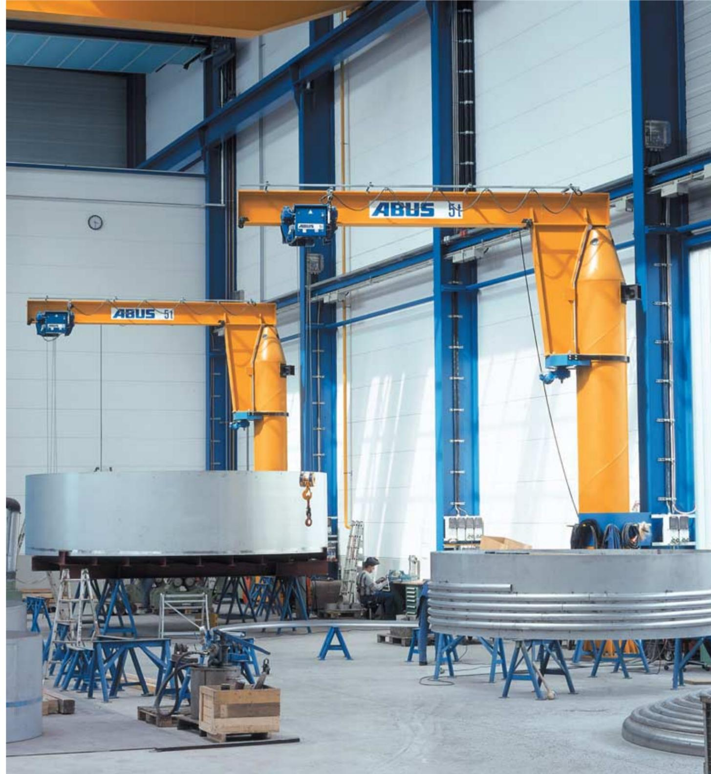
ABUS VS pillar jib crane with electric control of all crane functions used for brewing vat production (Huppmann).
