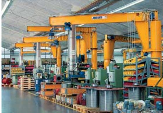
ABUS VS pillar jib crane used for assembling road milling machines (Wirtgen).
